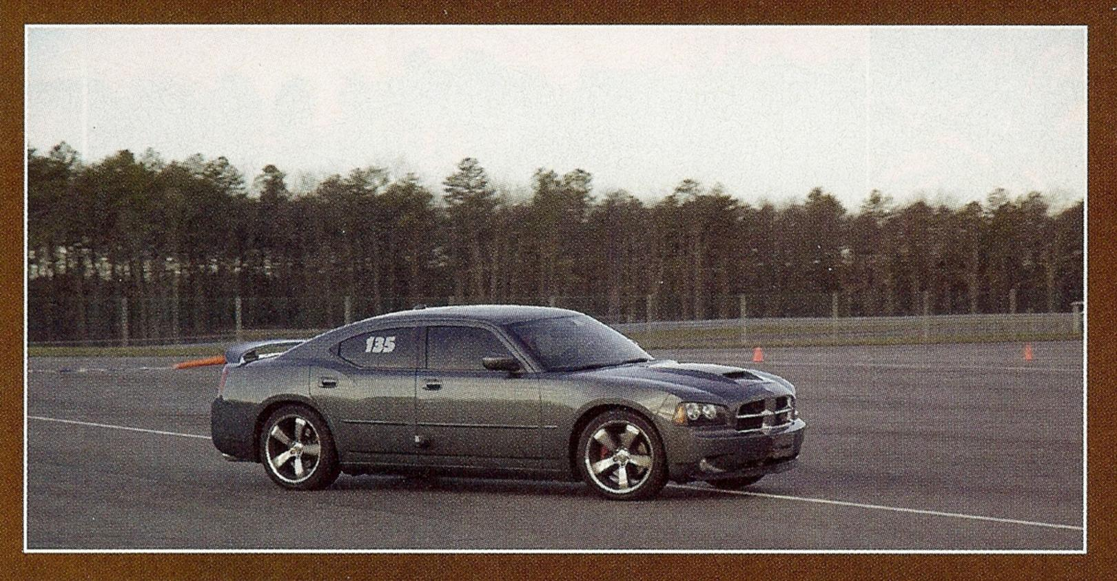
FOR COMPARISON, we rounded up a stock Charger R/T and ran it around the NJMS skidpad to a best of 0.87G. SRT8s are rated at 0.88G. Respectable, but there's definitely room for improvement.
